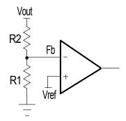
Figure 17 - Voltage Divider
