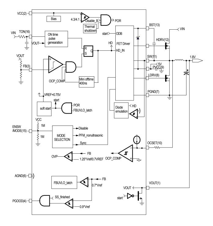
Figure 2 - Simplified block diagram of the NX2138
