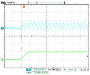
Fig. 14 Dynamic response in PFM mode (CH2 1.8V OUTPUT AC, CH4 OUTPUT CURRENT) VIN=12V, VOUT=1.8V
