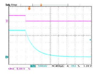
Fig.5 Turn off (CH2 1.8V OUTPU T, CH3 PGOOD)
