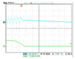
Fig. 15 Dynamic response in PFM mode (CH2 1.8V OUTPUT AC, CH4 OUTPUT CURRENT)
