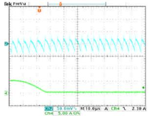
Fig. 13 Dynamic response in synchronous mode (CH2 1.8V OUTPUT AC, CH4 OUTPUT CURRENT)
