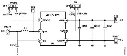
Figure 8. ADP2121 Evaluation Board Schematic
