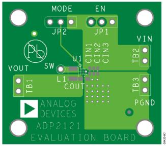
Figure 1. ADP2121 Evaluation Board Top Layer
