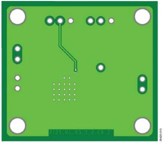
Figure 10. PCB Bottom Layer
