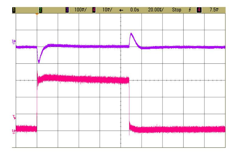
Figure 3. V<sub>OUT1</sub> Load Step Response
