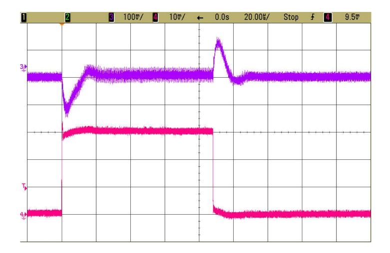
Figure 4. V<sub>OUT2</sub> Load Step Response
