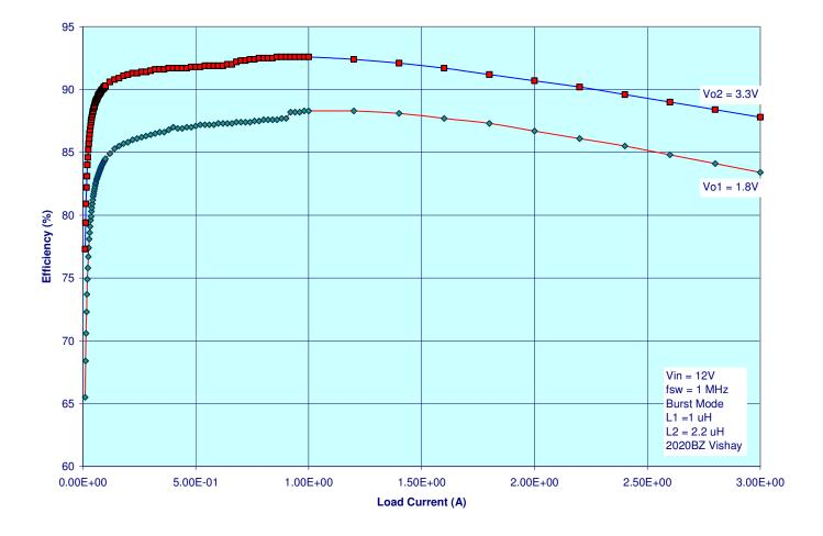
Figure 5. LTC3633 DC1347 Efficiency
