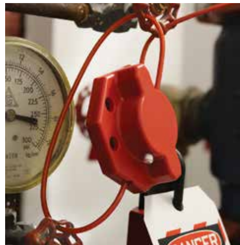
Turn the hasp halves to cinch cable.
