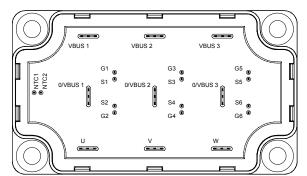
Pins NTC1 & NTC2 are only mounted on APTM100TA35SCTPG power module.
